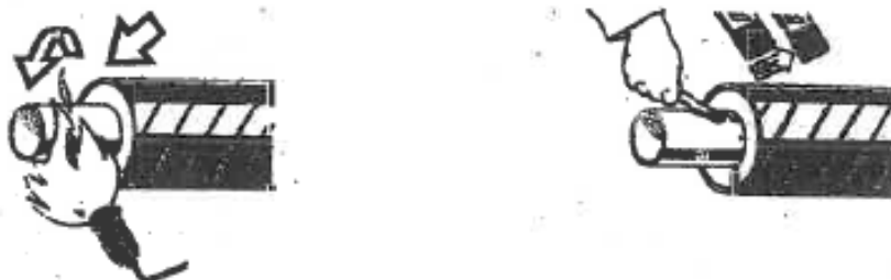
Heating of service (60°C) and casing (40°C) pipes
