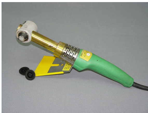
Photo No 8. Welding machine for plugs
