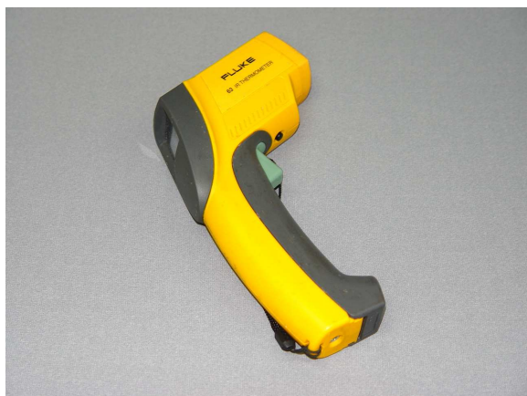
Photo No. 7 Pyrometer to measure the temperature of the heat-shrinkable sleeve - recommended
