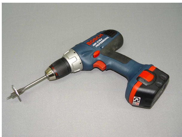
Photo No 9. Cordless drill with drill for drilling holes with a diameter of inlet 25 mm
