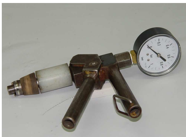
Photo No. 11 Test manometer with expansion cap
