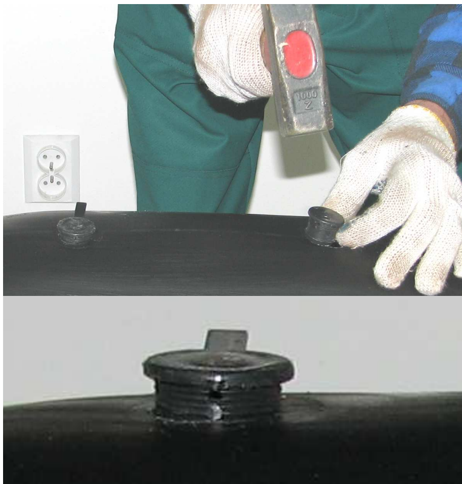
Photos Nos. 38 and 39 Embedding of vent plugs in the filling holes
